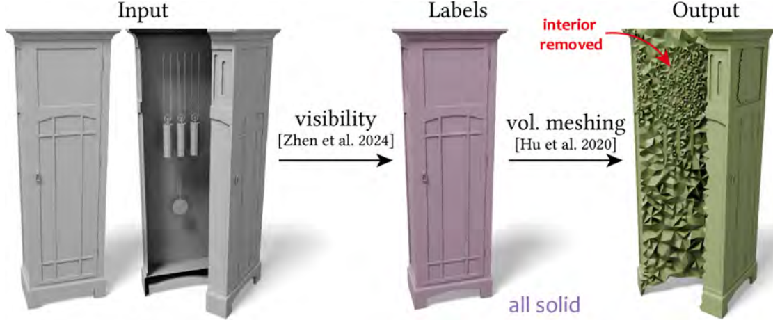
Figure 3.4: Existing heuristics, such as using triangle visibility [221], to classify solid/shell faces are prone to artifacts, such as deleting interior components.
