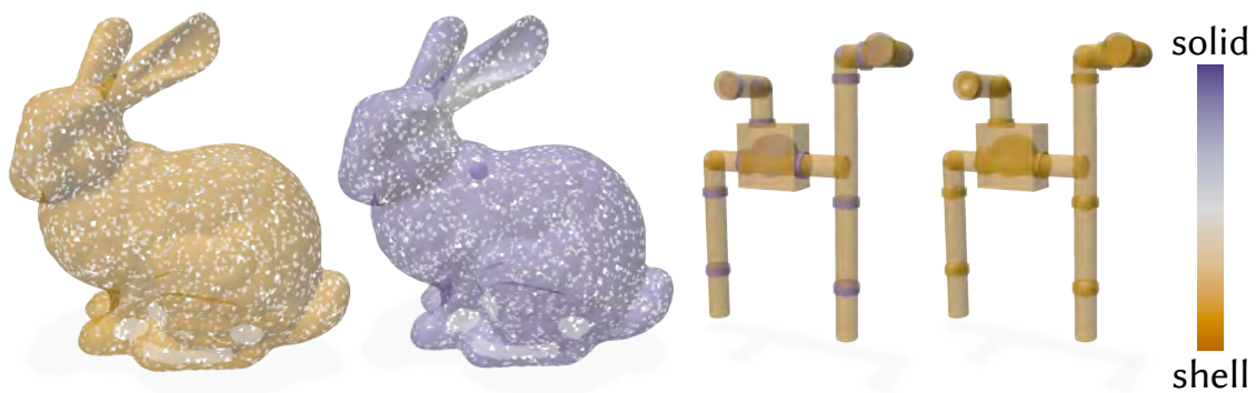
Figure 3.9: Left: A single constraint guides the optimization to classify a corrupted bunny (10 percent of faces removed) as fully solid. Right: A pipe modeled as a union of cylinders is classified as pure shell after placing some constraints.
