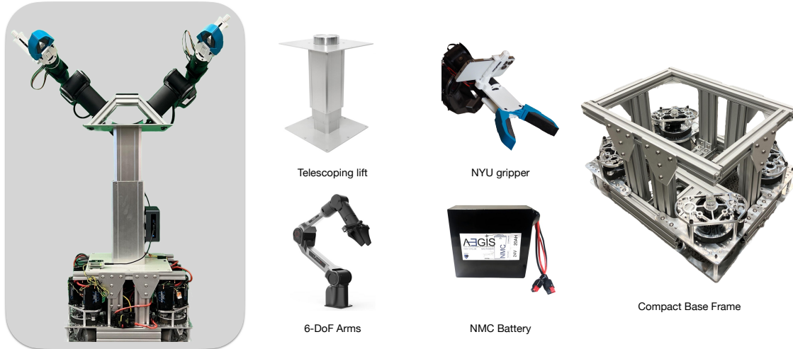
Figure 8.2: Cone-E is modular and easily customizable with different arms, end-effectors and sensors.
