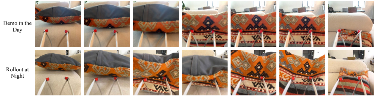
Figure 6.16: First person view from the iPhone from the (top row) Stick during demo collection and (bottom row) robot camera during rollout. The demonstrations were collected during early afternoon while rollouts happened at night; but because of the iPhone’s low light photography capabilities, the robot view is similar.
