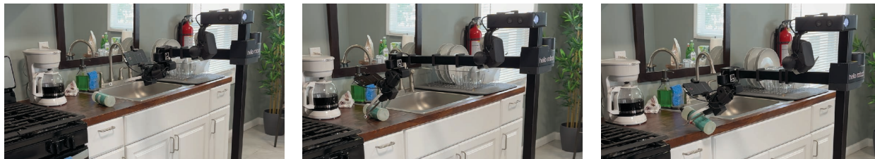
Reorientation failure: dropped bottle off the table, retry impossible
