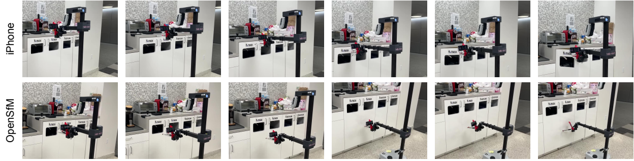
Figure 6.24: Open-loop rollouts from our demonstrations where the robot actions were extracted using (a) the odometry from iPhone and (b) OpenSfM respectively.
