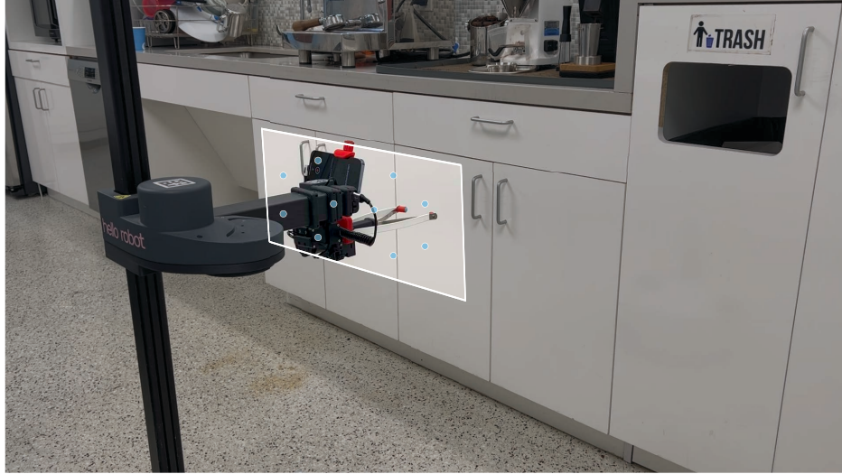
Figure E.1: 10-run evaluation schedule used to evaluate Robot Utility Models, with robot starting positions denoted by the pale blue dots in the image. We assume that the robot is at the task space facing the object, but it can be at different offsets with respect to the target object. On our object centric tasks (reorientation, bag and tissue pickup) we also randomize the position of the object itself.
