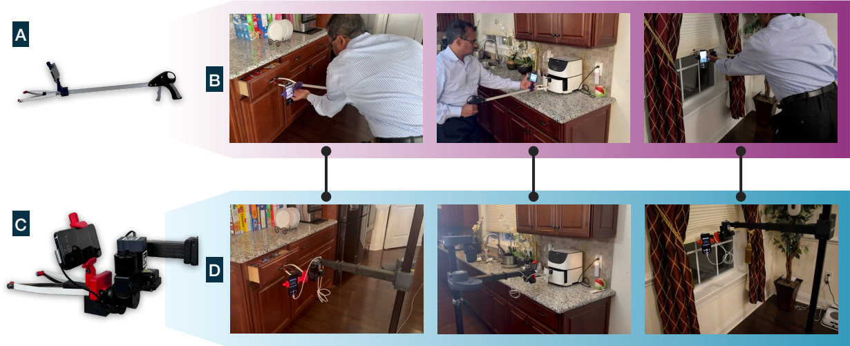
Figure 6.2: (A) We design a new imitation learning framework, starting with a data collection tool. (B) Using this data collection tool, users can easily collect demonstrations for household tasks. (C) Using a similar setup on a robot, (D) we can transfer those demos using behavior cloning techniques to real homes.
