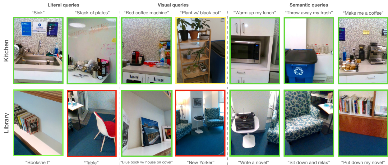
Figure 9.10: Examples of the robot’s semantic navigation in two different testing environments, looking at objects given different queries. The images show the robot’s POV given the associated query, with color coded borders showing approximate correctness. The rows show different two different scenes, top being in a lab kitchen and the bottom in our lab’s library/lounge space, shown in detail in figure 9.9.
