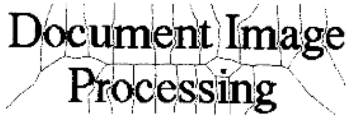
Figure 2.7: The area Voronoi region boundaries found for a small text region. Taken from [27]
