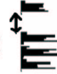
Figure 4.1: The width of the cut is identical to the length of the valley in the projection profile.
