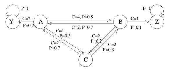
Figure 1: Markov process with final states
