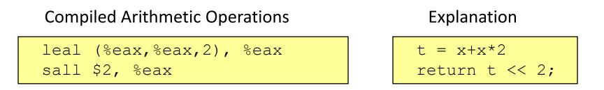
C compiler automatically generates shift/add code when multiplying by constant
