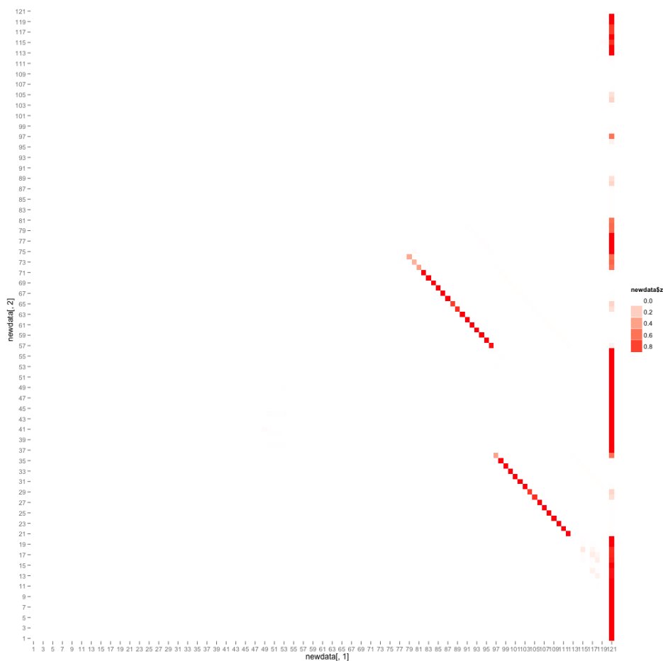
FIGURE 2.1. Heat-map plot of the probabilities of a pair of bases (i, j) binding in a stack containing two instructions, at its initial state. The length of the instruction's unique domain is 20 bases and the length of the clock strand is 16 bases. Thus, the total length of an instruction strand is 36 bases and the length of the complete stack including its three binding sequences is 120 bases. The entries in the last column, 121, correspond to the probability of the base i remaining unbound , so that it is equal to one minus the probabilities of binding to any other base in the complex. The ordering is done with the instructions first followed by the binding regions, as if we started counting with the first base of the last instruction to be unwound (the one appearing in black in Figure 1.1,) and went around in a clockwise direction on that diagram. In the heat-map, red denotes high probability and white denotes low probability. It is clear that the stack's sequences are such that the correct binding, depicted in Figure 1.1, occurs with very high probability, as the "stairs" match exactly the position of the binding strands hybridizing with the clock domains of the instructions. The bases in lighter red correspond to the first binding element, which has a slightly "frayed" ending.
