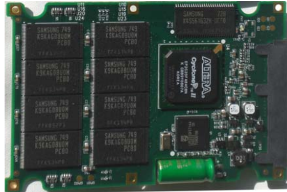
Figure 1: Internal view of the Memoright 32 GB SSD
