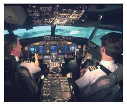
Using flight simulators, Boeing Commercial Airplanes customers are immersed in a realistic flight environment, enhancing their learning experience. Using computer-generated visuals to simulate surroundings, pilots can practice a variety of maneuvers related to high-risk situations without ever being in jeopardy
