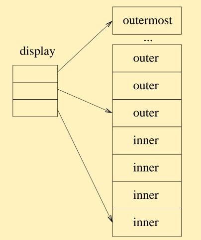
To retrieve entity n scopes out, need 1 indexing operation.
