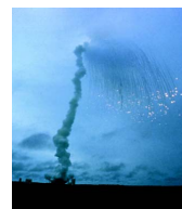
Ariane 501 failure (overflow)
