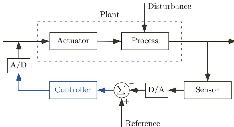
We advocate an approach in which code is generated by discretization both for the continuous dynamic nonlinear model of the controlled system (e.g. from the block diagram description of the plant, actuators and sensors) and for the digital implementation of the controller (as given by the control/command program to be verified).
