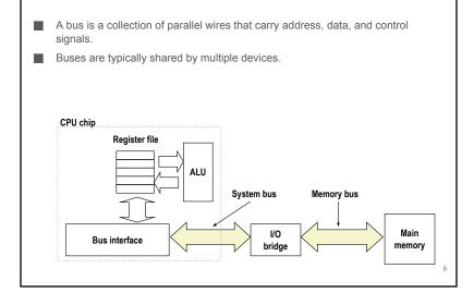
**Bus Structure Connecting CPU and Memory**
