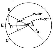
By construction we know that the length of line segment BD is a/2 and that angle A is 60 degrees. Hence angle a' is 30 degrees.
