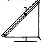
On a "Marconi-rigged" boat, the sail is attached directly to the vertical mast.
