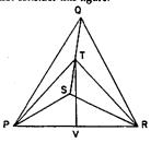
Here PQRS is a regular telrahedron with edges of unit length. T bisects edges QS and V bisects edge PR. Angle PTR is the dihedral angle between faces PQS and QRS. PT =  $\sqrt{3/4}$ , and PV = 1/2.
