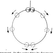
component. At the same time its downward acceleration increases, decreasing the force that it exerts upon the hoop. The maximum lifting force occurs when the sum of these two effects is greatest. Until the hoop actually moves, a bead does no work. Therefore, its gain in kinetic energy equals its loss in potential energy. Thus,  $(1/2)mv^2 = smg$ , where  $s = vertical\ drop,\ m = mass,\ g = gravitational$
