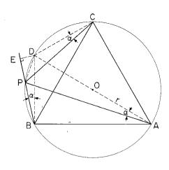
As can be easily proven, BD and DC, being the chords of a  $\pi/3$  arc, are equal to r, the radius of the circle AO. By our theorem, angle DPC =  $\pi/6$ . Since by our theorem angle DPB =  $5\pi/6$ , by subtraction angle DPE =  $\pi/6$ .
