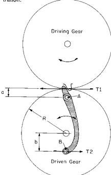
Both gears are the same diameter. The driving gear is conventional with teeth cut in the rim. The driven gear is a disc with teeth formed by levers supported by pins A and B. As both gears have the same diameter, input and output speeds will be equal. The driven gear will have the same tangential load (T1) as a conventional gear, but output torque will be increased by reaction of the lever on pin B producing an additional output torque (b · T2).
