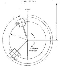
$\rho =$ liquid density, positive downward w = piston weight, positive downward s = piston stroke, from closed end; piston area = 1
