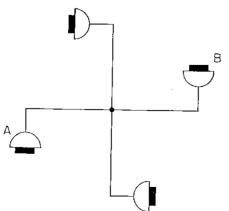
63 This "ferris wheel" is constructed under atmospheric pressure. Metal cups are attached to each arm, and a pliable membrane seals the top of each cup.
