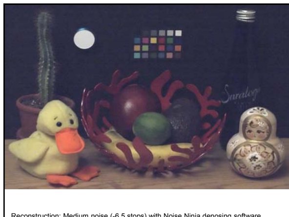
Reconstruction: Medium noise (-6.5 stops) with Noise Ninja denoising software
