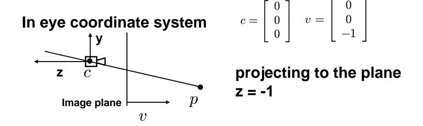
$$\operatorname{Proj}(p) = \begin{bmatrix} -p_x/p_z \\ -p_y/p_z \\ -1 \end{bmatrix} \qquad \operatorname{Proj}(p) = \begin{bmatrix} 1 & 0 & 0 & 0 \\ 0 & 1 & 0 & 0 \\ 0 & 0 & 1 & 0 \\ 0 & 0 & -1 & 0 \end{bmatrix} \begin{bmatrix} p_x \\ p_y \\ p_z \\ 1 \end{bmatrix}$$
