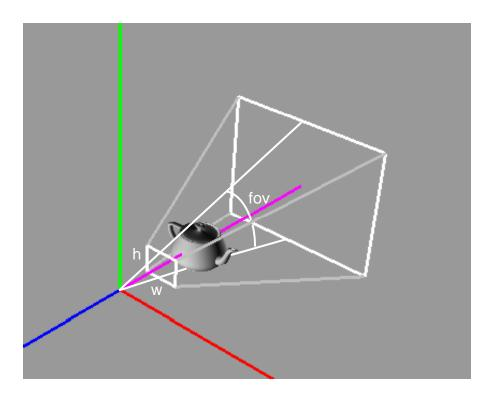
In the picture: fov = field of view, h/w = a=aspect ratio
