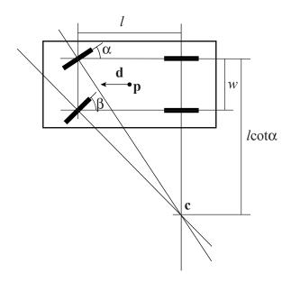
To do this we rely on the following general fact: at any moment in time, the motion of the car can be regarded as a rotation around a center (this center can be at infinity if the car is not turning).
