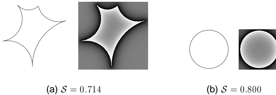
Figure 3.11. A highly concave shape (a) is “more convex” than (b) a circle, according to the measure from the decay process. The measure gives (a): 0.714 and (b): 0.800. Both shapes have the same area. ■
