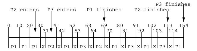
The diagram above is nearly self explanatory: The bottom column indicates the process that is running, with X signifying a 1ms context switches.
