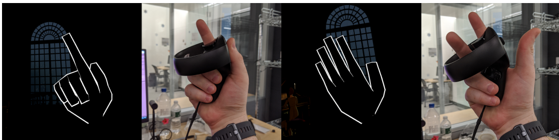
Figure 3.1: An example of mapping an Oculus Touch controller to an audience avatar. The images show that the hand mapping occurs using button states, instead of physical hand poses.
