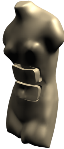
Figure 5.1: “Venus with drawers” (after S. Dalí) is created using union, intersection and difference operations.
