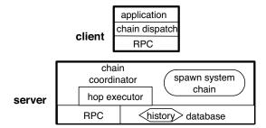
Figure 8: Lynx client library and server processes. The client dispatches chains using RPCs. The server process receives chains, queues them, and executes them against a local database. The server process also implements georeplication, secondary indexes, and materialized join views using system chains.
