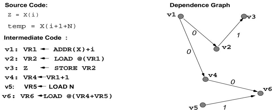
Figure 1: A Basic Block and Dependency Graph
