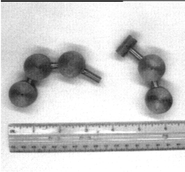
Figure 3: Prototypes of the mini actuator links for the legs of the Walking Machine.
