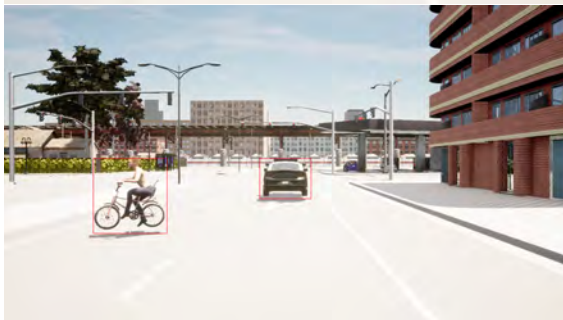
Figure 4.25: Interventions taken by the MLM. The first row is the original scene, the second after an intervention changing the police car to a biker, and the third after an intervention rotating the biker. The left side shows ground truth and the right shows model predictions. The model's predictions were very good for the first scene; in the second scene, it preferred a blank space on the left side to the biker, although the biker did get an 87% confidence. After rotating the biker, that confidence reduces to 34% while the model still hallucinates a vehicle on the left side with 95% confidence.
