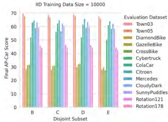
Figure 4.10: Test results with config 18C4 when training on disjoint IID subsets. Results are consistent, suggesting that the harder groups - bikes, rotations, and cybertruck - are ubiquitously hard.
