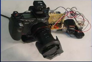
Ferroelectric shutter in front of the lens is turned opaque or transparent in a rapid binary sequence
