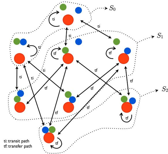
**Fig. 3.** Stratification of the configuration space induced by the contact constraints.
