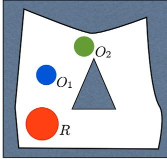
**Fig. 1.** Scenario of the considered manipulation planning problem. The robot  $R$  can autonomously translate in the plane while the movable objects  $O_1$  and  $O_2$  can translate only if in contact with the robot.
