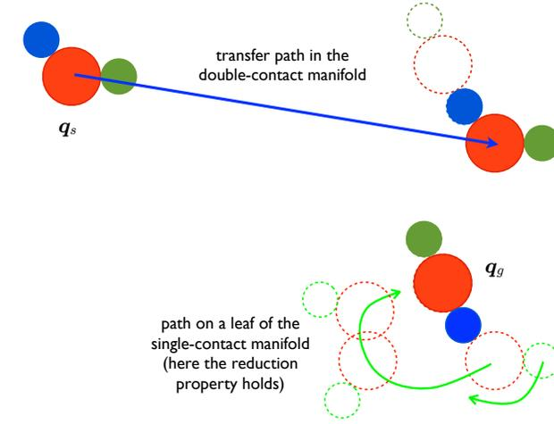
**Fig. 8.** Can any path in the double-contact manifold be “reduced” to a sequence of transfer and transit paths as in the figure?
