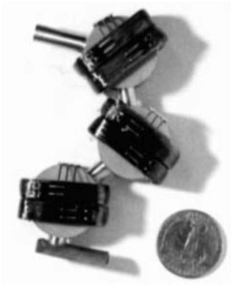
Figure 5.4: Prototypes of the mini actuator links for the legs of the Walking Machine built by R. Wallace and F. Hansen. (Photo by G. Kondogianis).
