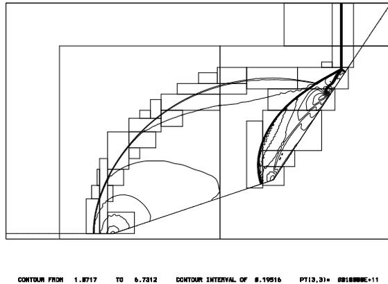
Figure 2: Time dependent shock reflection from a double ramp using h-box method with Cartesian grids. Density contours are shown.
