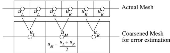
The coarsened grid integration step yields  $Q_{2h}u_M = u_M + \frac{\lambda}{2}(u_L - u_R)$ . Two steps on the fine grid for the cells adjacent to the jump yield
