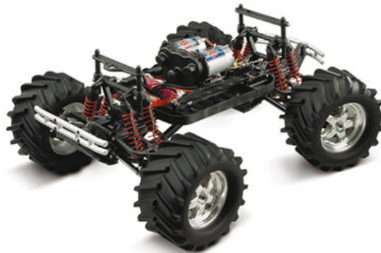
Figure 3. The chassis of the E-MAXX 1/10 th scale 4WD Monster Truck from Traxxas ( www.traxxas.com ).
