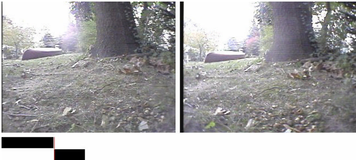
Figure 26. Example video images from the training data. The two pictures are taken by the two cameras at the same time. The two black bars below the images indicate steering wheel angle and throttle position of the human driver.
