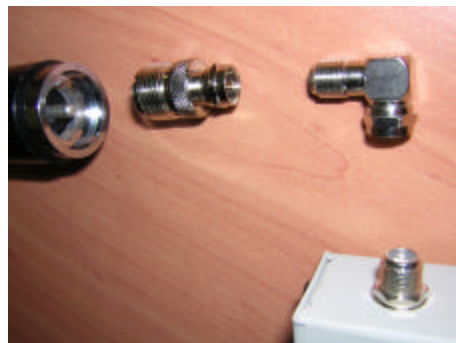
Figure 22. The connectors needed to adapt the UHF-style connector of the 900-Mhz antenna with the F-type input of the 900-Mhz receiver.
