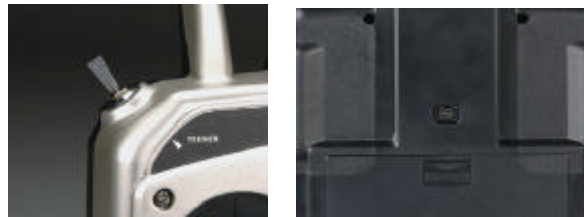
Figure 17. Trainer cord switch and connector on the Futaba 4YF airplane remote.
