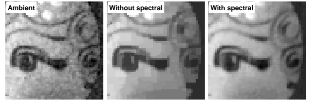
Figure 12: Close up of scene in Fig. 6 (top group) illuminated by candlelight. Left: Blue channel of white-balanced ambient shot, showing high noise due to lack of blue wavelengths in candle-light. Middle: Denoising of ambient using likelihood and spatial priors only. Right: Denoising of ambient using spectral constraints from the red and green channels, in addition to the likelihood and spatial priors. The spectral constraints significantly improve performance.
